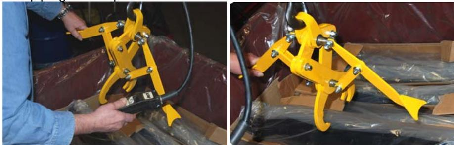
Step 4: Grasp the object. Lift one of the pipe guide weldments to open the grab (photo 5), and while open, lower the grab around the object (photo 6). Lower the pipe guide weldment until the load-engaging portions of both arms (identified in FIG. 1) contact the top of the load material (circled in photo 7).
