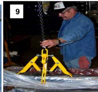
Step 7: Lower the load to the ground/supporting surface (photos 11 and 12). Position the object above the surface that will receive it (ground, pallet, work platform, etc.). Make sure that the load is not swinging or rotating before beginning to lower it.
