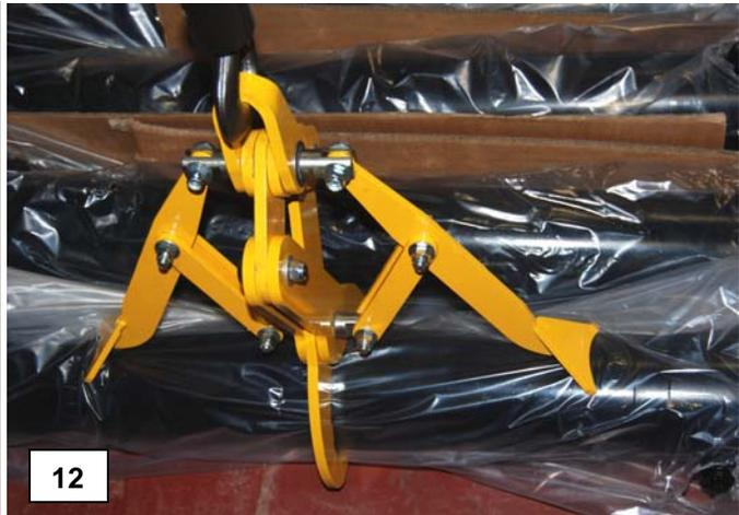
Step 8: Once the load has been fully lowered, immobilize it. Disengage the pipe grab by lifting one or both of the pipe guide weldments. Raise the grab so that it is completely free of the load.
